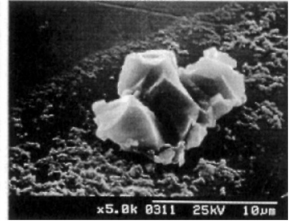
Wear particles formed by transgranular (left) or intergranular (right) fracture of silicon nitride.
